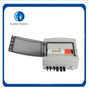
GD-PV4/1 combiner box is suitable for inverter (MAX input voltage DC550V/DC1000V,2PV input channel, 1 output channel, single MPPT inverter). Box body is made of PVC engineering materials,with test for fire retardant, Temperture rise,anti impact, anti ultraviolet, and other testing. IP65 protection grade.
