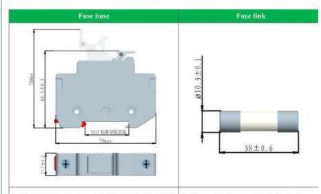
1. **Shell:** PBT environmentally friendly plastic, 100% raw material pressed, with excellent electrical properties and heat aging resistance, flame retardant grade V-0;
