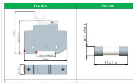
1. **Shell:** PBT environmentally friendly plastic, 100% raw material pressed, with excellent electrical properties and heat aging resistance, flame retardant grade V-0;
