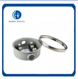
100A,120/240V AC,single phase,2 or 3 wires, Line and load lugs:1/0 Max,Cu-Al Conforms to ANSI12.7 Mounting : Surface, pole outdoor Locking: Sealing ring has lock provision
