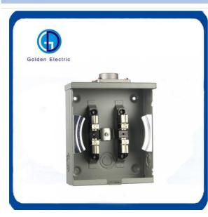
100A/125A,600V max, Single phase, 2 or 3 wire Conform to ANSI12.7 Heavy duty tinned copper jaw NEMA 3R type construction 1.2mm thickness(#18 gauge) galavanized steel sheet. Ample gutter space for easy wiring The fixed hub size 1/2" to 2-1/2" for option
