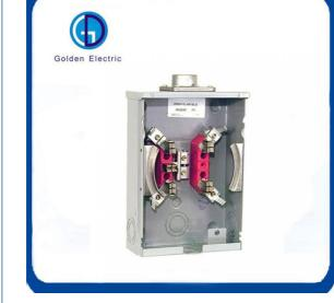
200Amps,600V AC. Connector ine and load size #6-350 Cu-Al Heavy duty tinned copper jaw with reinforce clip C/W center netural bar NEMA 3R type construction 1.2mm thickness (#18 guage) or 1.5mm thickness (#16 guage) galvanized steel sheet, electrostatically applied epoxy baked gray powder finished. Ample gutter space for easy wiring Convenient knockouts in the side back and bottom Lay in type terminal with pressure plates for easy connections The fixed hub size 1/2" to 2-1/2" for option
