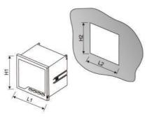
面框尺寸(mm): L1xH1 开孔尺寸(mm): L2xH2 Frame size(mm): L1xH1 Hole size(mm): L2xH2
