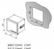
面框尺寸(mm): L1xH1 开孔尺寸(mm): L2xH2 Frame size(mm): L1xH1 Hole size(mm): L2xH2
