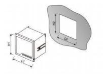
面框尺寸(mm): L1xH1 开孔尺寸(mm): L2xH2 Frame size(mm): L1xH1 Hole size(mm): L2xH2
