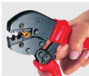
先把端子按规定的压口放好 Put the terminal in relevant die set firstly
