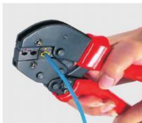
只需稍稍施加两手的压力就能完成压接 Press gradually and crimping well
