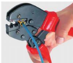
接着把已剥皮绝缘导线放进端子 Then put the stripped insulated conductor into the terminal
