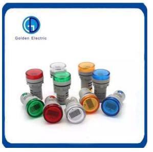
Color: red, green, yellow, blue,orange & white Voltage: 6V-380V (Customized available) Current: ≤20mA Panel mounting hole: 22mm Temperature: -20°C - +50°C Average temperature: < +35°C Humidity: <50% (+40°C<) & <90% (+20°C<) Power Supply: AC ,DC , AC/DC
