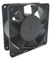
General Specification: Frame:Aluminum Alloy Impeller:PBT(Black)UL94V-0 Operating Temperature:-10°C~70°C Motor Protection: Auto Restart or Polarity Protection Insulation Resistance: 20MΩ or over with a DC500V Megger Dielectric Withstand Voltage: AC500V 1s
